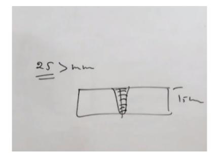
So normally it is applied when the plates of greater than 25 mm thickness to be welded. The plates up to like say the 15 mm thickness can be welded directly in single pause without ash preparation using the square group. So direct in one go the things can be brought to the molten state through thickness penetration can be achieved for the welding purpose.
