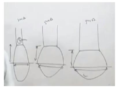
Now, I will talk about little bit the bead geometry aspects like for a given current, for example, 100 ampere current being used using these 3 different electrodes say one 2.3 electrodes we are using say 3 mm size, 4 mm size and 5 mm size electrode. So the size of the arc like this, like this and like this.
