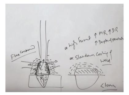
So, whatever the power is fed that is very efficiently and effectively used. So why it is so, in this case the electrode is fed through the rollers using say, then here is arc this is our work piece say, the plates to be welded and here the contact tube will be feeding the current to the electrode and here see all around this one will be a pool of the flux is mount or piling up of the flex is done. So, whole of the arc is actually submerged under the flex.
