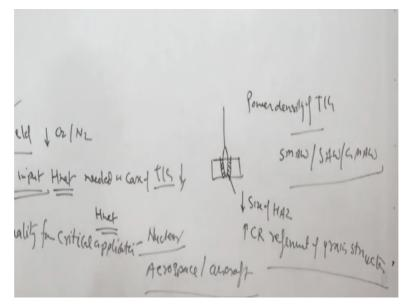
And because of these reasons in addition to the effective, in addition to the capability to produce clean weld, in terms of the low concentration of the oxygen and nitrogen, the TIG offers another unique feature or ability among the arc welding process, that is capability to melt with very low heat input. So the net heat input, which is needed in case of the TIG process. This is very less as compared to the other process.
