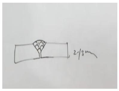
So in this case what we need, the process may work in case of thin plates, the process may work without any filler like thin sheets can directly be joined using the autogenous approach like plate of the 3 mm thickness, these are the two plates. It can by application of the TIG arc we can directly fuse them together and after the solidification will be getting the weld joint.
