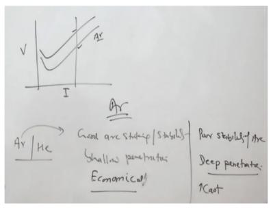
So sometimes water cooled torches are used as far as this GTW process is concerned. So the torch is another member and they are also categorised based on the kind of current that they can handle as I said, 3 to 200 ampere or 5 to 300 ampere, or much higher, so high capacity current capacity torches are water cooled. So another thing is about the shielding gas. Shielding gases are commonly used are argon and the helium.
