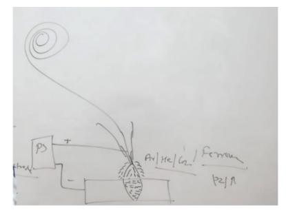
So here you see, the electrode wrapped in its pool feds through the cables to the nozzle and then through the nozzle, it comes out the shielding gases will also be coming out. And here the electrode develops the arc between the work piece mostly in this case, the power source connected to the positive terminal of the power source is connected to the electrode and negative is connected to the work piece.
