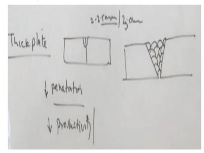
But the gas Tungsten arc welding process suffers with the one major limitation and that is, since the process, here like in case of the welding of the thick plates it offers the two kinds of the problems, one is normal GTW process offers the maximum penetration around 2-2.5 mm or in very severe condition very high heated condition may be 3 mm in single pass. So GTW
