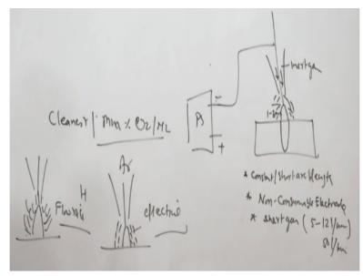
So now I will talk about the reason behind why it offers the cleanest weld means with the minimum percentage of the oxygen and nitrogen in the weld. So here, the schematic of the system with like this, we have power source positive and negative terminals. So negative terminal is connected to the electrode, say this is electrode, Tungsten electrode and here is the work piece.
