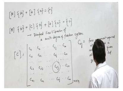
And we find represented in terms of matrices, so it was M x double dot + K x = 0, so this is this equation is for an undamped spring mass system multi degree of freedom system. now if we have damping and we introduced the damping in the system we have the C1 C2 C3 terms, then one more matrix will come into this equation and we call it damping matrix so we will we can write, so this is equation of damped free vibration of multi degree of freedom system.
