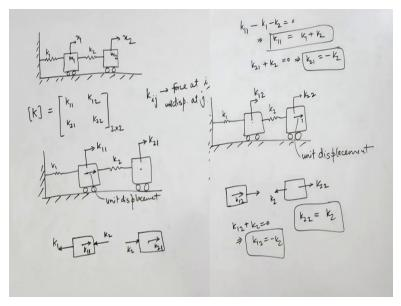
So we have this two degree of freedom system consisting of two masses m1 and m2 and to stiffness elements k1 and k2 now we have to find the stiffness influence coefficients and so the stiffness matrix K so it will have k11, k12, k21 and k22, because it is two degree of freedom
