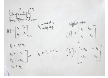
So we have obtained the all the four influence coefficients stiffness influence coefficients that is k11 that is k1 + k2, k21 that is -k2, k12 - k2 and k22 = k2, so again from here we see that k21 = k12 = -k2 due to the reciprocal theorem. Now we can write our stiffness matrix, so now we see that how we can find the stiffness influence coefficients for multi degree of freedom system and how the reciprocal theorem.
