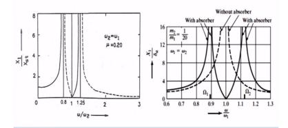
So these 2 natural frequencies; for example, if we have earlier omega/ omega 2 = 1, now we have at 0.8 and 1.25. So these are the 2 natural frequencies and we can see that, we can see that when we start any machine, it is start from some low speed and it raises to; its operating a speed. Therefore, if it passes through the lower resonance frequency of the system for example here, if it passes through 0.8, although its operating frequency is here.
