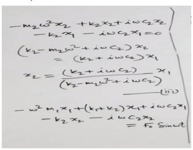
Now we can put these values of x1, x1 dot, x1 double dot and x2 x2 dot and x2 double dot in equations 1 and 2 and we can find; we can solve for x1 and x2. So if we put; so let us put it,
