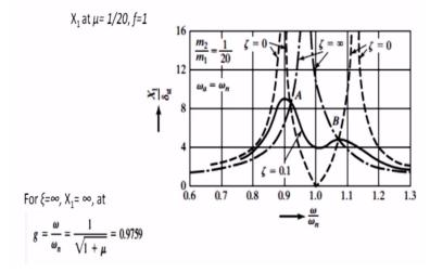
And here we can; for some given mass ratio 1/20 and f=1, we can see that for zeta =; so this is this equation is plotted for zeta = infinite and zeta =0, so we see that the; for zeta = infinite, x1 is again infinite and corresponding g is 0.9759. Okay, so it means the; for 0 damping, the x1 is infinite. Because without 0 damping means there is no any damping in the system and we are getting these natural resonance frequencies.
