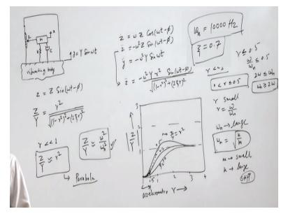
so we have this system, so this is our vibrating body, so this is vibrating body or vibrating structure. So this is vibrating with some Y=Y sign, omega T, and we are placing the seismic instrument here so seismic instrument has some stiffness and damping element. And then it has some seismic mass, M, K and C and of course seismic mass will have some X and here we will have Z and we have this frame and here we have some scale.
