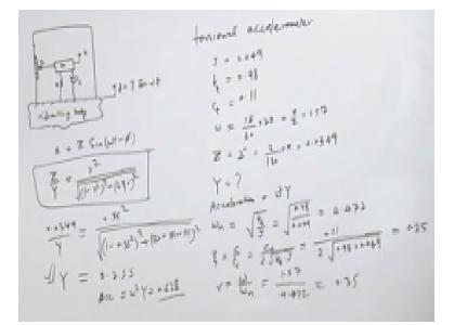
So, it is coming about 0.255 and so omega square y that is excitation amplitude and so we can take omega 1.57. So, it is about 0.628. So we can see how to calculate these acceleration values for any system. Here we have considered the torsion system. Okay, so we stop here and thank you for attending this lecture and see you in next lecture.
