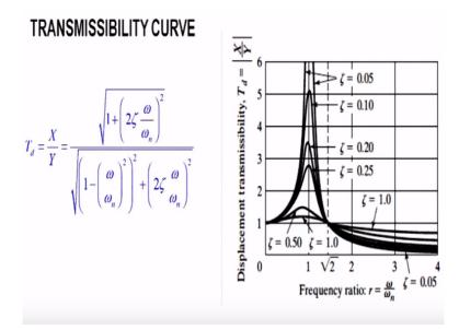
So here we can see the transmissibility curve again for the displacement transmissibility. Of course, the curve the nature of the curve will be same as, we obtained in the case of force transmissibility. So here again we see that the curve we start from one at R = 0 and it goes to Maximas near, r = 1 and again it drops and passes cross the transmissibility 1 or = 1 at under root 2.
