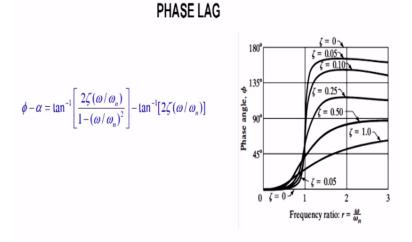
Similarly, if we see the phase lag, so phase lag, this phase is starting from zero and for Zeta less than 0.5, it is going to some maxima and then coming and tending towards 90 degree while, for Zeta > 0.5 there is no maximas but directly they are increasing to 90 degrees for r greater than for higher values of r okay. So now we will do one problem based on the displacement transmissibility.
