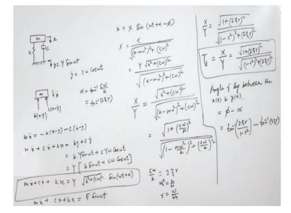
So we have a mass and here we have we say this is the support, but this support has some motion, it has some motion. So okay, so the support is moving, it is vibrating, so this is a case of the support similar the case of the support vibration and we can do the analysis, by making the free body diagram of this mass. So, this is the mass and we have, because this spring will be compressed by x - y.
