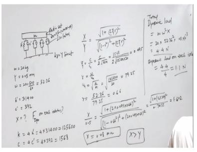
So, we have a radio set, So, it is like this system, so we have this is a radio set and it is put on four isolators, so we have four isolators okay. So, we have four identical isolators here, and this in mass m this is radio, so this is a radio set, and these are our isolators. So, four identical Isolators and each has some k and let us say k dash and c dash some values each, so m is given 20 kg and the  $y = y \sin Omega t$ , so y is given 0.05 mm and then it is 500 cycles per minute.
