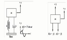
So, we can see that, this motion transmissibility also we call it displacement transmissibility. So, it is the ratio of the amplitude of the response x to that of the amplitude of the support okay. So, let us see here there is some sensitive instrument m is kept on some surface ok, and that surface is vibrating with some harmonic way and so this motion is going to affect the response of this mass.
