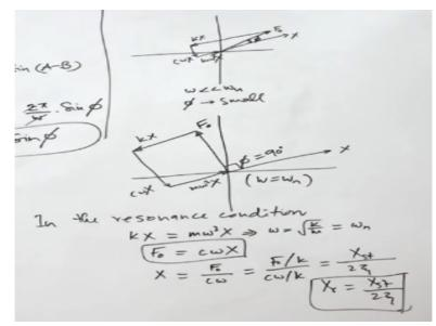
Now we take some cases here, if we remember the vector diagram that we made for the forced harmonic vibration of a single degree of freedom system. So we have this vector diagram, here this is x and this was F0, then this is kx, this is c omega x and this is m omega square x and this is phi. So if we see while omega is much less than omega n, the phi is very small and in this case, so omega is very less.
