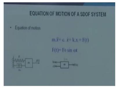
So there could be random force on the system like the force of the wind or some earthquake, they are random. So these are the mainly four type of forces but out of these, we are going to concentrate on the harmonic force. So we have a single degree of freedom system, single degree of freedom system that comprises mass element, stiffness element and damping element.
