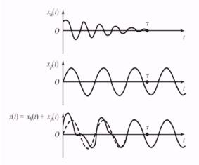
And these part is a harmonic function with sin function and this is the steady state part and these part will prevail even after this part is 0. So we can show the response of a single degree of freedom system, so here; we see that the first part is shown the complementary function xc or xh here it is, so it is going to decay with time so here it is like free vibration, so it is going to decay with time and this is the particular integral part that is harmonic sinusoidal.
