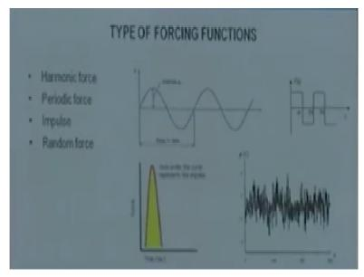
And the system vibrated with its own natural frequency. In case of forced vibration, when we say forced means, that is force applied to the system and what will be the response of the system? What will be the frequency of vibration of the system in these conditions? So this will be the subject of this lecture. So let us discuss the type of forcing functions, so what are different type of force that or loads that can be applied to the system.
