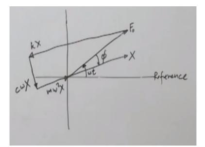
So these 4 forces, we can represent on a vector diagram, because they are the forces, they are vectors, we can represent them on a vector diagram. So let us make the vector diagram. So when we want to make the vector diagram, first we plot the x in the direction of x; first we plot F0, because F0 sin omega t, so from here it is omega t, this is the reference axis, so it is omega t F0.
