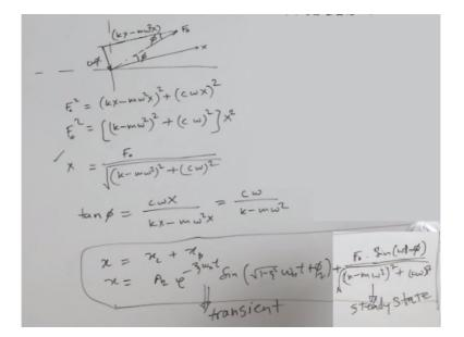
Now we can write these; so we can make this vector diagram even better like, so we have x, this is F0. So we can write, like this is kx and this is m omega square, so this quantity is kx - m omega x square x and this is c omega x, so here we can write F0 square = kx - m omega square x is square + c omega x square. So here we can write k - m omega is square, whole square + c omega whole square x square = F0 square.
