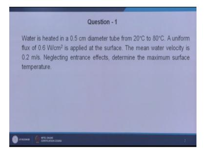
Let us say we are having water which is being heated in a water is being heated in a 0.5cm diameter tube, so tube is having 0.5cm diameter from 20° to 80°. A uniform flux of 0.6 W/cm<sup>2</sup> is applied to the surface of the tube okay. So that means you have a uniform heat flux case over here okay. The mean water velocity is 0.2 m/s and you have to neglect the entrance effect, so
