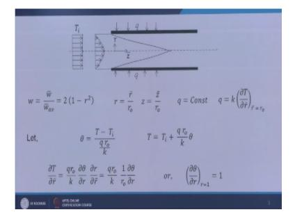
So let us go inside this first I will be showing stigmatically what situation we are going to study in this so as I have mentioned we will be having a tube so this is a tube having center line this one are coordinate is radial coordinate is in this side okay and this is axial coordinate in this side okay and here we are considering thermally fully developed profile, so that means parabola boundary condition and there we are considering that in the tube we are giving constant heat flux.
