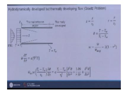
So let me start with this schematic so here we will be considering hydro dynamically developed but thermally developing flow, usually this type of problems are called Greetz flow okay Greetz problem we can call okay. So here you see this is our pipe line let say here we are having the center line okay, here we are having the center line and now somehow the velocity boundary layer has developed and had taken actually a parabolic profile okay.
