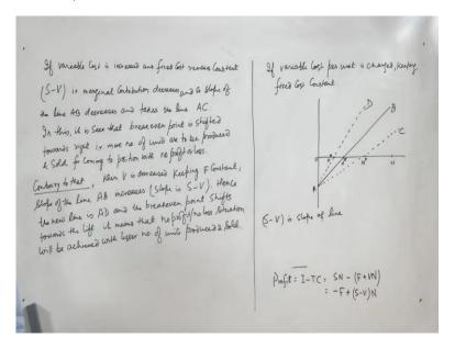
So your x axis is cut at this point and your breakeven point is shifted towards left. So we can write these things, so if variable cost is increased and fixed cost remains constant S minus V, that is marginal contribution decreases and so slope of the line AB decreases and takes the line AC.
