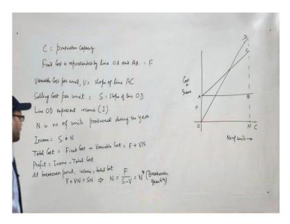
The fixed cost is the one which does not depend upon the number of units produced and the variable cost will be changing with the number of units produced. So if this is number of units produced and if this is the cost or income, in that case there is a fixed cost line and also there is variable cost per unit line. Now we have an income line which goes like this. Now in this suppose the organisation has a capacity that is C. So C is the production capacity.
