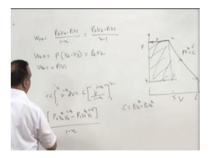
And that turns out to be work under during one to two that turns out to be P2V2 - P1V1/1-N because here in this process work is consumed by the system we will take negative of this and the final expression will be and this expression is for the work under this curve. Let us say 5 and 6, so work under 1, 2, 5, 6 this is the work done during compression from state 1 to state 2 for state 2 to state 3 is going to be P2V2 - V3 because V3 is 0 we can always write P2V2.
