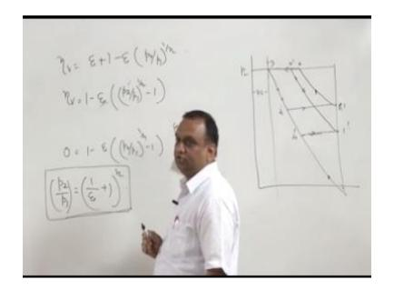
If you look at this expression if the pressure ratio is high if the pressure ratio is high it is going to affect the volumetric efficiency and volumetric efficiency will reduce. If you increase the clearance ratio if we increase the clearance ratio or clearance for say VP the volumetric efficiency of the compressor will reduce. But in any case in a refrigeration system approximately 5% of clearance ratio is maintained. It can go up to 7% but minimum of 5% of clearance ratio is maintained.
