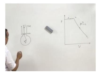
Most of the applications in vapour compression system it is a vertical type of system. So there is a crank case and a cylinder and piston is fitted inside the cylinder. So when the crank rotates with a certain rpm to inflow motion of the piston takes place their two positions that is top dead center and bottom dead center where the direction of the movement of the piston, the change in the direction of the movement of the piston takes place and this length is known as stroke of the compressor.
