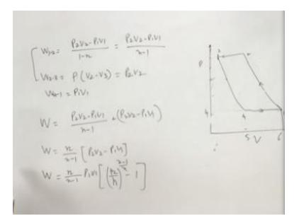
So piston will be striking the head of the cylinder therefore in order to avoid any damage to the head some clearance is provided, and this volume is known as clearance volume. So after the compression process remains same from state 1 to state 2, but instead of reaching up to here the stroke terminates at state 3 and some clearances provided between the piston head and the cylinder head.
