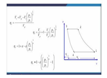
So V1 is clearance volume plus VP and V4, V4 we can take as clearance volume multiplied by P2 by P1<sup>1/n</sup> this is this expansion process. The index of compression is from state 1 to state 2 is n and we have assumed that index of expansion is also n, however it may be different also. So this is V1 - V4 expression for V1 - V4 and expression for V1 - V3 is VP only. Now if you simplify this we will be getting VC/VP + 1- VC/VP P2/P1<sup>n</sup>.
