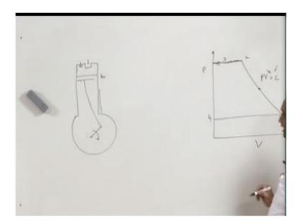
What happens I will draw a larger diagram, what happens when the piston moves in upward direction the system behaves as a go system it has two walls this compressor has two walls initially both the walls are closed. So when compression takes place it follows the polytrophic equation up to state 2, the moment the pressure 2 is attained exit walls opens, when the exit wall opens the vapor inside the cylinder is removed at constant pressure.
