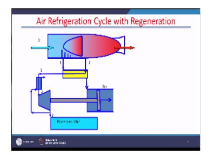
After the strain three there is a heat exchanger this heat exchanger as shown in the figure takes air after the expansion of turbine so part of the air after the expansion of turbine it is re-circulated through this heat exchanger so that the temperature of air is further cool to state four. (Refer Slide Time: 04:44)
