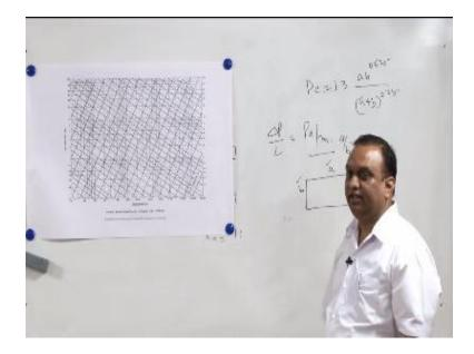
And these friction losses starting from 0 point 1Pascal meter to 100 Pascal meter 100Pascal meter is very high friction loss, similarly to length liters per second are also very high discharge rate so high where and the vertical lines here it means vertical lines in this chart vertical lines in this chart are from our for air quantity constant air quantity horizontal lines are the pressure constant pressure drop this chart is for friction chart for round ducts.
