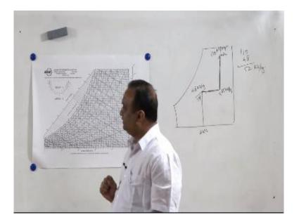
Now we will draw a horizontal and vertical line and we will get A state A this will be in the form of sensible heat and latent heat. So air which is coming into the room shall bring energy in the form of sensible heat and this is latent heat and this is sensible heat addition by the air. Now if I calculate these values, now from here then this enthalpy head of the air which is at 40°C temperature and 50% relative humidity is approximately 110kj/kg.
