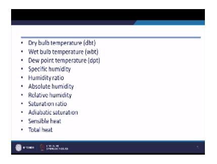
Now absolute humidity and relative humidity, ratio suspicion humidity ratio absolute ability absolute humidity, is the mass of water vapour associated per unit volume, so it is on volumetric basis, absolute ability nowadays it is not used as a parameter. Ready humidity is important it is used everywhere, in fact in order to express the state of moisture in the air rating this term relative humidity is used.
