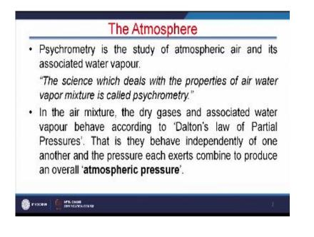
Psychrometry is the study of atmospheric air and its associated water vapor so thermodynamic study on this the mixture of pure air and the water vapor is known as psychrometry and psychrometry is very helpful in air conditioning processes, because in air conditioning normally
