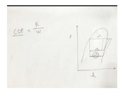
Now efficiency of air conditioner, now in a refrigeration system you where using CoP coefficient of performance, co-efficient of performance was refrigerating effect divided by energy spent for this refrigerating effect that is energy consumed by the compressor, the same CoP is used for air condition also every year the conditional has certain CoP, now in air conditioner normally CoP is air than the refrigeration system.
