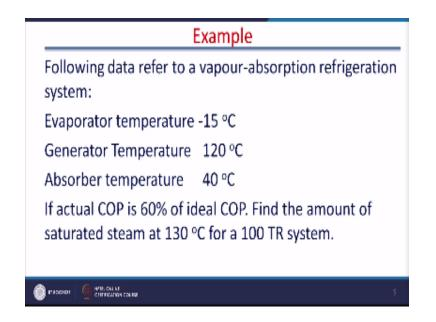
Suppose for absorption refrigeration system the following data referred to vpour absorption refrigeration system where.
