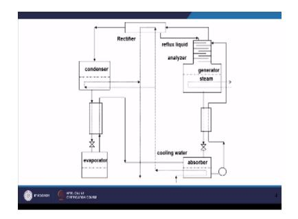
Now I will draw arrangements in a ammonia water refrigeration system so we will start with the absorber.
