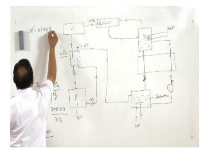
COP' it is 60% of this it becomes 5727, here 10 TR of refrigeration system has to be given so 10 TR means sorry, 100 tonnes of refrigeration so 100 tonnes of refrigeration means 100x3.5kW this much of energy is required and this much of energy is required for this steam at 130°C suppose steam is used for heating at 130°C we can assume that steam is condense here and mass of the steam is the energy supplied and that so mass of the steam can be calculated as.
