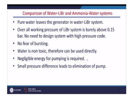
So overall working pressure lithium bromide system is barely above 0.15 there is no fear of bursting because the pressure is very low water is non toxic therefore can be used directly. Negligible energy for pumping is required here for the purpose of pumping negligible energy is required. Small pressure difference leads to elimination of pump, if the small pressure difference there we can swap these cylinders and in that case the pump can be eliminated.
