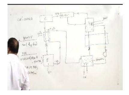
You know COP is refrigerating effect that is 100x3.5 and mad mass of the steam multiplied by hg-hl I mean enthalpy of saturated steam so m=350/COP is 05727 multiplied by 2720.8-546.38 this is 2720.8 is the enthalpy of saturated steam at 120°C and this is enthalpy of saturated liquid water at 120°C and this gives the mass value has mass flow rate as 0.28115kg/s or mass flow rate is 16.87kg/m. So this is the amount of a steam which is required here to produce  $-15^{\circ}$ C temperature here.
