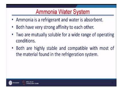
Because they are very strong affinity to each other water and ammonia two or mutually soluble for a wide range of operating conditions is specially existing inside the system both are highly stable and compactable with most of the material found in the refrigeration system except copper, copper is not compactable with ammonia so wherever ammonia is used copper fittings are not used. (Refer Slide Time: 02:48)
