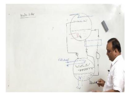
Water lithium bromide absorption system where water works as a refrigerant, now this is the high pressure vessel this is the low pressure vessel. In high pressure vessel suppose water vapour is condensed in high pressure vessel we will start from condenser so there is a pooling water I will show with a blue ink so it will be easy to understand, so this is water chill water which flows here and water vapour is condensed and water vapour is collected in this tray.
