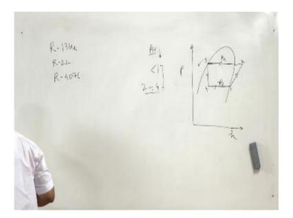
As you can see in a PV diagram mostly heat transfer takes place during phase change of refrigerants either boiling or condensation this is pressure. So 1, 2, 3, 4 refrigerating effect is attained here and that is due to phase change. During this process also condensation of refrigerants takes place.
