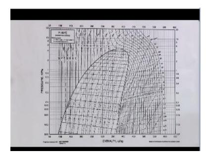
For the more clarity, I will show you the ph diagram of 4:07 C you can see this is the saturation line, saturation curve on y-axis pressure on a log scale on x-axis, there is a enthalpy at on a linear scale, there is a thick saturation line, on the left hand side there are vertical lines constant temperature line and constant temperature lines, are inclined they are not horizontal.
