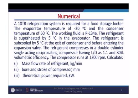
Now we have mass flow rate of refrigerant with us with this mass flow rate of refrigerant we can always find the power consumed inside the compressor and with this mass flow rate we can also find the size of the compressor. Now in order to find the dimensions of the cylinder as we have to find in this numerical bore and stroke of the compressor. So first of all will calculate the swept volume of each compressor that is  $\Pi$  by 4 D<sup>2</sup> square into stroke of the compressor.
