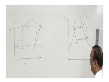
The temperature entropy the process on temperature entropy diagram that is PS A B C D sorry this direction this direction and if the liquid is sub cooled here is superheated here, so if the vapor is superheated here it will be like this A will be shifted here and if the liquid is are pooled here we assume it to be along the this liquid layer but actually it is somewhere here it is compressed liquid and expansion takes place like this.
