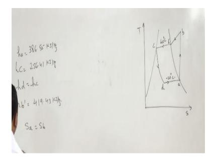
So vapor is saturated before entering the compressor that is state A then state B T superheating condensation and then expansion and then we get CD, B1 and this is temperature here it is entropy the direction of process is like this temperature is 40 degree centigrade that is and this temperature is minus 20 degree centigrade HA here again we can take directly from the properties table then HA is equal to again 386.55 kilo joules per kg.
