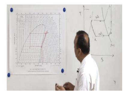
Now if I want to transfer these processes on pH diagram let us take the processes one by one, temperature entropy super heating saturated then expansion. so A b c d x = 1, x = 0 state 1 and this is 40 degree centigrade and this is minus 20 degree centigrade, now here at state 1 minus 20 degree centigrade saturated vapor we can directly take enthalpy from here state be 40 degree centigrade saturated vapor.
