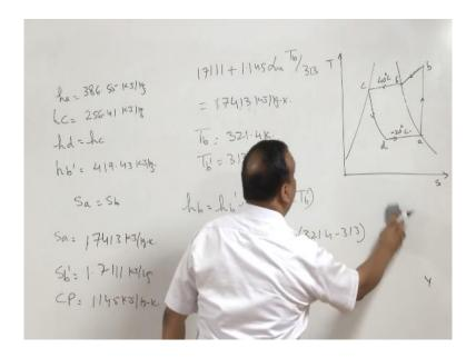
Change in entropy Delta s is going to be equal to 1.145 natural log PB/ 313 and this change in entropy plus entropy at state B dash will give if we add this Delta s to entropy at B dash the entropy at B dash is 1.7111 + 1.145 natural log PB/ 3 1 3 we will be getting entropy at A, entropy at A is equal to 1.7413 kilo joules per kg Kelvin, if you solve this and the value of PB is going to be 321.4 Kelvin.
