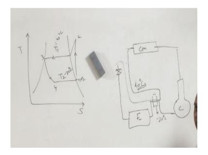
Where the vapor enters from evaporator it goes to the compressor from compressor it goes to the condenser, condenser and from condenser it goes to the expansion valve expansion were from expansion valve to the evaporator if we depict this process on temperature entropy diagram it is going to be like this, so one two three and four and this is temperature t1 and this is temperature T2.
