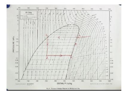
Now if I want to use pH diagram for this now in this pH diagram forty degree centigrade the vapor is saturated at the entry vapor is saturated here, now vapor that is state A now vapor is compressed it is isentropic compression and the pressure in the condenser is constant so we will follow A light which will follow the closest constant entropy line and perhaps we'll be getting A point B somewhere here point B somewhere here.
