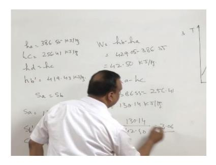
And that is going to be equal to 386.55 - 256.41 and that will give you 130.14 kilo joules per kg because mass flow rate is one kg per second so if you multiply this by 1kg per second we will be getting 130.14 kilowatt now CoP of the system 130.14 / 42.50 = 3.06.
