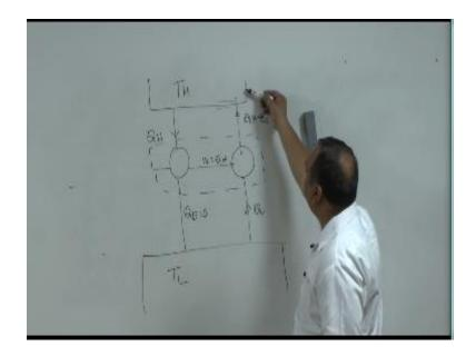
$Q_H$  amount of heat is taken, and work is done by in the  $Q_H$  amount, and zero heat is rejected to the reservoir, this is violation of the Kelvin –Planck statement, now we have a device which is pumping q amount of heat, and if we connect this with this device instead of having output on this side, if we couple them then this is going to be  $W = Q_H$ , and heat transmitted to the high temperature reservoir will be  $Q_H + Q$ .
