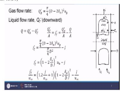
So this is Qg` and liquid flow rate would be Qf`. So Qg` can be written as the area occupied by the liquid sorry, gaseous plug multiplied by the velocity of the gas. So here what we have considered the pipe diameter was D and we have considered that this thickness of the film uniform thickness of the film around the gaseous plug is D infinity. So overall we will be finding out the diameter of this gaseous plug is D-2\*delta infinity.
