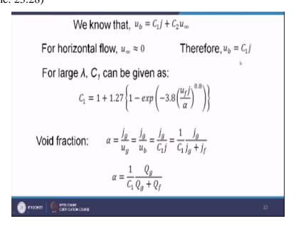
So here what we can do, u infinity we can make 0 because it is in horizontal pipeline. So there will be no velocity, unconstraint velocity of the bubble. So you can write down u infinity = 0. So we get ub= C1j, over here C1j right. Now once again various correlations are there. 1 very important correlation is for finding out the C1 for horizontal slug flow C1 will be 1 + 1.27 {1- e to the power (- 3.8 (ufj / sigma) to the power. 8)} right.
