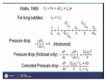
So we can find out that volume of the bubble will be v \*alpha and this volume of bubble, this volume can be written as a into ls + lb. Now this A\* ls + lb is the volume for the (()) 25:26 width of the cell. Whatever we have shown over here that we are having a gaseous plug and liquid slug. So if you consider a unit, so this unit volume is this 1 A is the pipe diameter and ls is the slug length and lb is the bubble length.
