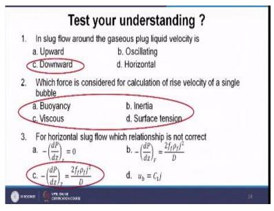
First, in slug flow around the gaseous plug liquid velocity is 4 options we are having upward, oscillating, downward and horizontal. So mostly you have understood what is the answer correct. Answer is downward because liquid will be having downward velocity around the slug. Okay second question which force is considered for calculation of rise velocity of a single bubble okay.
