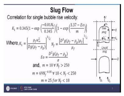
And in between 2 gaseous plugs, we will be having liquid slug. So in real slug bubble regime you will be finding out lots of satellite bubbles are here proceeding this gaseous plug but for simplicity and purpose of analysis we have eliminated those satellite bubbles. We are only dealing with the gaseous plug over here and followed/ A liquid slug.
