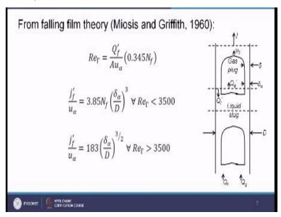
But I will be showing that how empirically can be found out using falling film theory how the liquid velocity superficial velocity can be found out. So here you see this velocity will be nothing but jf /u infinity will be 3.85 Nf. Nf already we have discussed that is non-dimensional inverse viscosity into delta infinity, uniform film thickness / D whole cube. This expression valid is valid for Reynolds number, film Reynolds number less than 3500.
