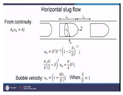
Once again the same situation this is having bubble velocity. The film thickness we have represented as delta okay. And here I have shown the length of the bubble as lb and the length of liquid slug as ls. Now if you start from the very basic continuity equation then I can write down Ab to into ub = A\*j. Why because you see in this horizontal slug flow actually the movement of the bubble will be causing the overall flow because otherwise it is not assisted by buoyancy.
