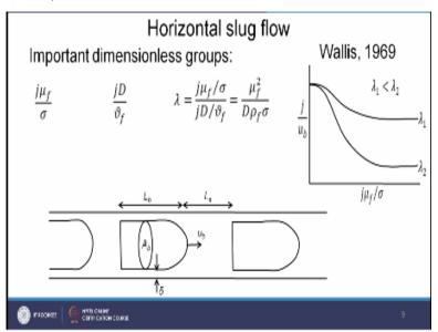
So important non-dimensional numbers first one is jMu f/ sigma okay. Second one we can take as jD/Mu f. So this is having the viscous effect this is having the surface tension effect compare to viscous effect. And another one we can derive as lambda which will be the ratio between these 2 okay. So here you will be finding out that in this we are having 3 parameters lambda, jMu f/ sigma and jD /Mu f.
