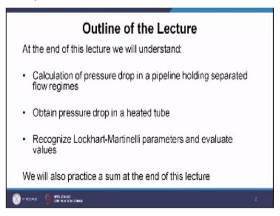
So at the end of this lecture we will understand the calculation of pressure drop in a pipeline holding separated flow. So basically, we will be giving you how to calculate the pressure drop as we have shown you in case of homogeneous flow. We will obtain pressure drop in a heated tube. So from the adiabatic situation will be converting into heated tube situation. So heat is coming from the periphery of the tube.
