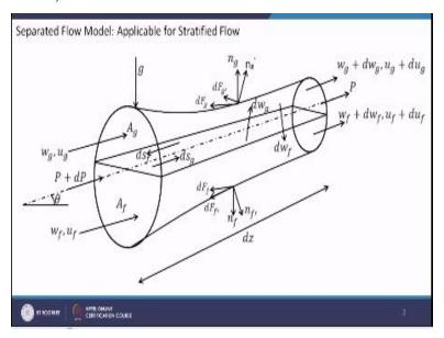
So basically, you can find out separated flow is applicable for situations like stratified flow so here I have shown you a stratified situation for liquid and gas. So liquid is at the downward side and gas is at the upward side. And here to make it generalized we have considered the pipe is changing its diameter as well as we have considered that this is making some angle with horizontal which is theta right.
