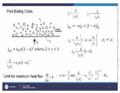
So as we are having the heat flux so we can find out the lots of bubbles will be generated over here. Bubbles will be moving up and liquid will be coming down for replenishment right. So we are having 2 different situations over here bubble velocity up and liquid velocity down. So we have taken jf, jv and jl into consideration. Now this jv is signifying the vapor gaseous phase. We have written here as jg and liquid phase jl we have written here as gf.
