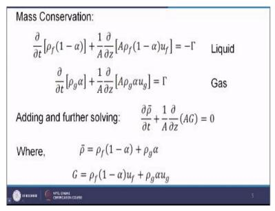
So you can find out this the unsteady part which we have already seen in our fluid mechanics. So this is the unsteady part delt/ delt t [Rho f (1- alpha)] and then we are having the inertia part 1/A delt/delt z [A Rho f (1- alpha)uf. So (1 -alpha) is coming into picture as we considering the liquid part. Now this - gamma is actually due to the mass transfer. So some liquid is converting into vapor due to phase change.
