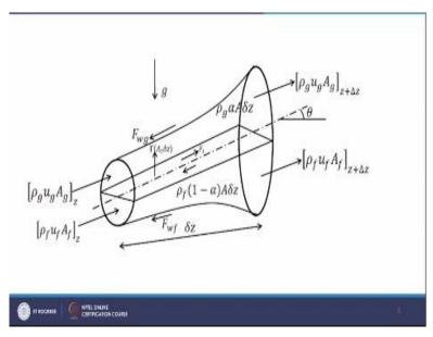
We can find out this is smaller cross section compared to this 1. So we are having variable cross section and to show the relative velocities between the phases we have considered both phases are separate. So you see at the bottom we have given liquid phase and at the top we have given the gaseous phase. So liquid phase is signifying f and gaseous gas phase is denoted by g. So you can find out that the as the flow is flowing from left to right.
