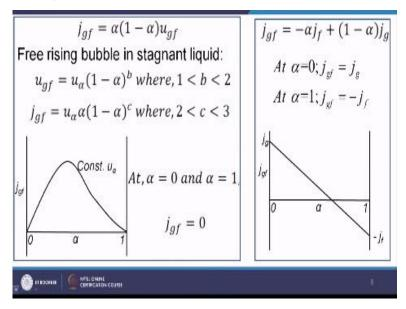
So you can find out first equation which I will be using jgf = alpha (1 - alpha) ugf okay. Now if we talk about bubbly flow situation that means lots of bubbles are there. We will be finding out that Ugj is actually a function of velocity of free rising bubble okay. So you can write down that
