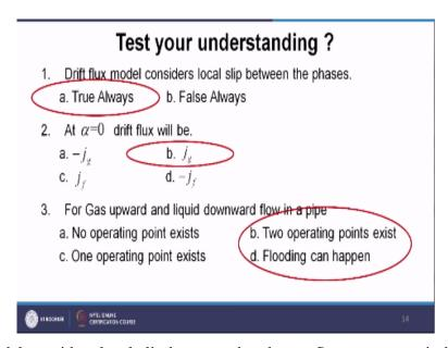
So drift flux model considers local slip between the phases. So you answer in between true and false obviously the correct answer will be true always. Next at alpha equal to 0 drift flux will be jgf will be 4 options were having – jg, jg, jf, - jf the answer is jg. Then for gas upward and liquid downward flow in a pipe we are having 4 options, no operating point exist, 2 operating point exist, 1 operating point exist and flooding can happen.
