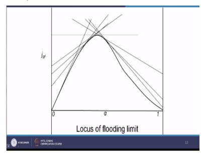
You have to do the experiments for different liquid velocity and gas velocities that means jgf = jf, jg at alpha = 0 and equals to -jf at alpha = 1. And we can find out this type of flooding limit points and if we find out the low cause of this flooding limit that will be the curve right. Next let us try to see another important case which is called pool boiling crisis.
