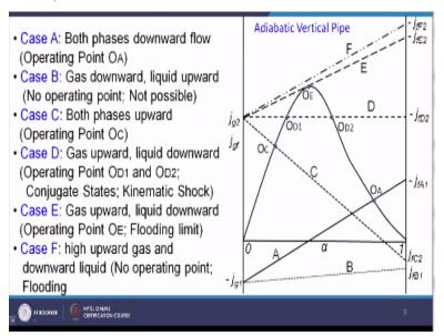
You know we have shown you in the previous slide. So it gets 0 over here. At alpha = 0 and alpha = 1 right. Now let us take several cases. So first one we will be taking case A, which is both the phases are having downward flow. So you if both the phases are having downward flow that means both jg and jf they are negative. So if they are negative then will be finding out at alpha = 0. Negative sides we need to go for jgf = jg so that will be becoming minus jg1 right.
