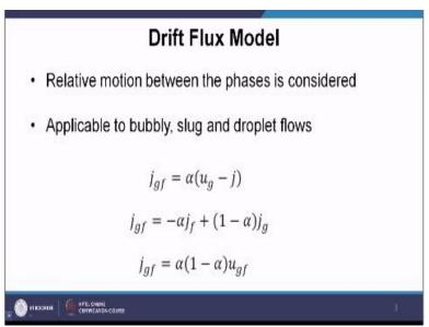
Basically, we will be finding out drift flux model is applicable for bubbly flow, slug flow and droplet flow. So, wherever interface is not clearly distinct just like your bubbly flow and droplet flow and its immediate transition slug flow. We will be finding out drift flux model is applicable.
