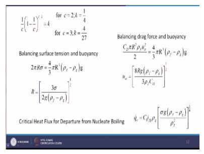
Then to obtain the final value of the critical heat flux let us balance the drag force and buoyancy. So if you balance the drag force and buoyancy so you will be getting this is the drag force cd \*pi / pi r square \* Rho f \*alpha square/ 2. And this is the buoyancy 4/ 3 pi rq with the volume multiplied by density ratio into g. So you will be getting the terminal velocity u alpha in this fashion where r is also there.
