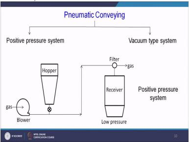
Next let we see, let us show you that what are the different types of gas-solid flow. We see in industry, in industry those gas-solid flows are mainly observed in pneumatic conveying line. So you will be finding out the pneumatic conveying line gas and solid are coexistently flowing with each other.
