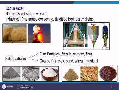
Some of them are pneumatic conveying, fluidized bed and spray drying okay. So here I have shown some examples experimental and numerical examples where gas-solid flow is occurring in industry. Now there are different types of solid particles which can coexisting gas okay. Depending on the size of the particles we define them as fine particles and coarse particles.
