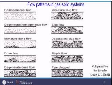
Then you will be finding out degenerated homogenous flow. You can find out the homogenous flow is actually becoming a heterogeneous one, low towards the lower side lots of particles are being dumped and then immature dune flow somewhere the some shot of dune type you can find out. But that is immature that has not taken its usual shaped.
