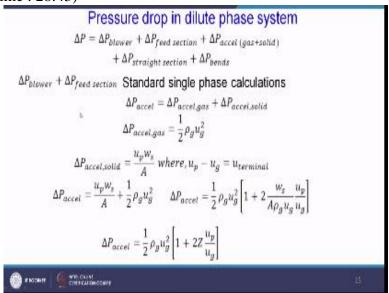
Then let us try to find out what does the pressure drop in a dilute pipe value phase system okay. So pressure drop delta p will be actually dependent on the component whatever I have shown you delta p will be delta p blower + delta p feed section. Wherever feedings will be the hopper then you will be having delta p acceleration due to gas and solid + inside the pipeline you will be having acceleration pressure drop.
