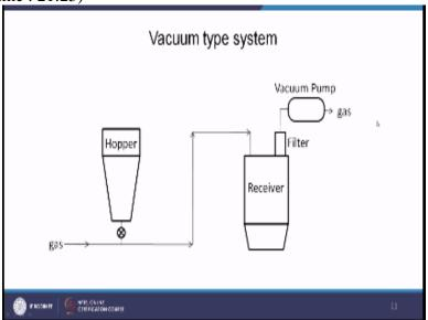
Then next one, let see the vacuum type. In vacuum type, you will find out that though the gas is coming over here and taking the particle from the hopper but it is not actually driven by positive pressure of you know blower in place of that what you have given at the end of the receiver. You have given a vacuum pump which is actually dragging the air from atmosphere through this pipeline okay. And you know at the end of this one receiver will be collecting this particle.
