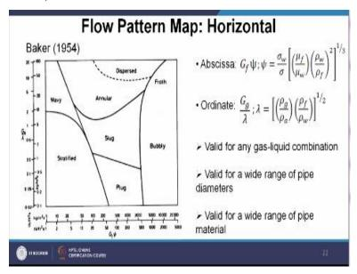
You can find out once again all those flow regimes. Whatever we have seen in horizontal stratified, wavy annular froth, bubbly, slug, plug all these flow patterns you can find out. This is also applicable for any horizontal gas liquid Two Phase Flow. So in the abscissa we have given gf \*psi. So gf \* psi is an abscissa and gj into by lamda is in the ordinate.
