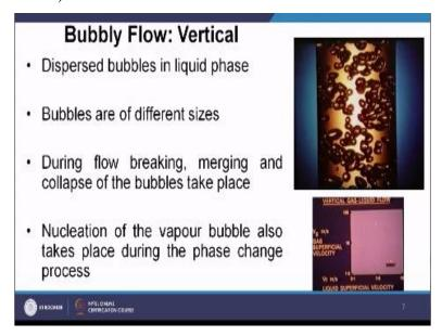
You can see this video, so lots of disperse bubbles you can see in the liquid phase. (Video Starts: 08:52) One important observation is that the bubbles are of different size okay and bubbles are causing breaking merging and collapse. So sizes are changing whenever it is moving upward. You can see nucleation of the vapor bubbles also takes place over here due to phase change. So, smallest size of bubbles will be generating in this phase. (Video Ends: 09:13)
