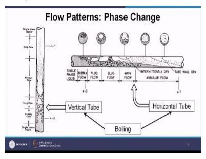
So you can find over here that we have shown 2 different situations vertical tube and this is a horizontal tube. You can find out we can, we are starting from singe phase liquid and we are giving heat around this tube. So, lots of bubbles are being generated at the pipe, pipe wall via nucleation. Those bubbles are getting bigger over here in size and finally forming a slug bubble which is resembling a slug flow.
