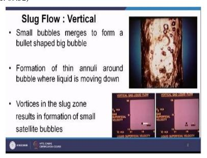
Here, we will be finding out small bubbles of bubbly flow those are merging and forming a big slug. (Video Starts: 10:01) Okay, so bullet shaped big bubble which is actually a slug bubble being formed over here. I will be showing you in the figure you can see this is a very big bullet shaped bubble followed satellite bubbles. So you will be having vortices in the slug zone which will result the formation of small satellite bubbles also right.
