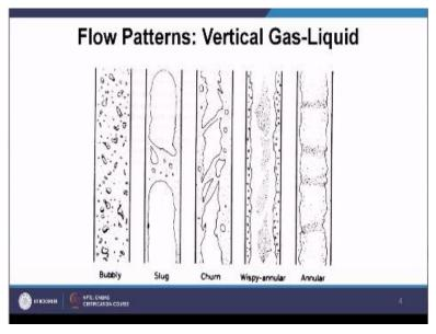
So see it is starts from very tiny dispersion of gaseous phase in the liquid one. This type of flow regime, we call as bubbly flow. So here separate identity of individual gaseous phases is not there. So you can find out a homogeneous mixture of gaseous phase in the liquid. So this is characterized by small bubbles.
