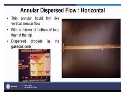
(Video Starts: 15:28) So in case of annular dispersed flow you can find out over here that thick annular liquid film is there okay. This is the film you can find out over like a vertical annular flow whatever we have seen in the previous slides okay and this film is thick at the bottom and thin at the top. So we can find out here we are having thick film and here we are having thin film.
