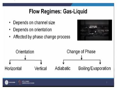
The orientation of the channel whether it is vertical or is it horizontal it will be affected by phase change processes. So if there is some sort of phase change process definitely this will be affected by phase change. Now in case of orientation, we know there will be horizontal and vertical position and in case of phase change we will be having adiabatic and or in case of presence of phase change we will be having boiling or evaporation.
