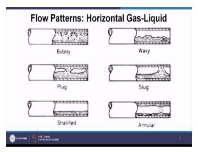
First one is as usual bubbly flow but it is interesting to note the bubbles are not well dispersed in the pipeline. Most of the time, the bubbles are sticking with the upper side of the channel okay. Same phenomenon applies whenever these bubbles actually merges and forms a plug flow over here. So plug flow is nothing but a big gaseous slug formed by merging of these bubbles. So you will be finding out the plug flow over here.
