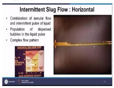
(Video Starts: 17:38) So, here what you will be finding out this is actually combination of annular flow and intermittent pulse of liquid. So we can find out first this is annular flow and then there is pulse of liquid with lots of bubbles entrapped inside this. So this is very complex pattern and this population of dispersed bubble in between these will be causing the flow pattern very, very interesting to see.
