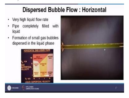
(Video Starts: 17:00) So if you increase the liquid superficial velocity further. So you will be finding out that pipe is completely filled with liquid okay here you can see completely filled with liquid okay. Formation of small gaseous bubbles were at the top somewhere over here you can find out the gaseous phase bubbles okay.
