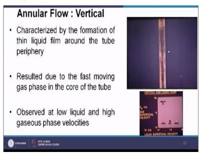
(Video Starts: 11:38) So this is a close view at high speed so you can find out here we are having film and the periphery, at the center we are having the gaseous phase. So this is resulted due to fast moving gas phase in the cross section also you can see this is the liquid film and in the core you are having gas phase only. Okay it is observed actually at low liquid and high gaseous phase.
