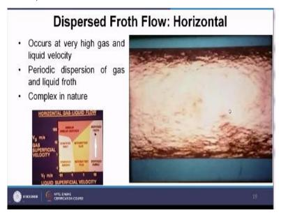
(Video Ends: 18:22) So from dispersed bubble flow if you increase the gas superficial velocity, you will be coming to this dispersed froth regime. So you can find out over here that we are having period of dispersion of gas and some liquid froth over here. In the cross section we can observe that one this is also very complex in nature studying this one requires lots of idea about the bubble dispersion as well as interfacial phenomenon (Video Ends: 18:48).
