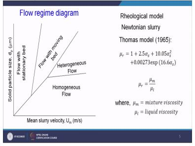
Let us try to see; now how we can characterize these flow regimes depending on the velocity, mean velocity of the slurry and the particle diameter, because these are 2 important parameters on which the regime will be depending. So let us see over here. So here you see in the abscissa we have plotted the mean slurry velocity and in the ordinate we have plotted the solid particle size dp. So you can find out over here whenever the
