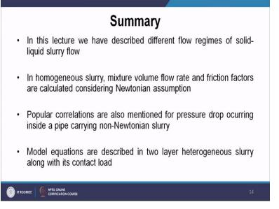
So let us summarize in this lecture. We have described different flow regimes of solid liquid slurry flow. In homogeneous slurry we have found out the pressure drop considering laminar, turbulent and considering Newtonian and non-Newtonian slurry. And finally for heterogeneous slurry using 2 layer model, we have shown how pressure
