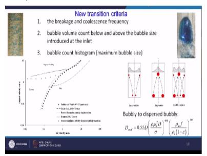
Then using this model 1 new transition criteria also. So you see whenever we are getting a bigger size bubble that is very much flow into slap bubble shape and go to the slug flow regime. So far that we have given new transition criteria so that can be constructed so depending on the breakage and coalescence frequency.
