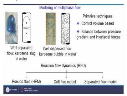
So you see over here, this is the kerosene Taylor bubble in a slug flow followed by some small kerosene bubbles over here as satellite bubbles okay. And in the second figure, you see we have given lots of small kerosene bubbles well dispersed in the water boundary okay. So if you compare these 2 then you will be finding out that in case of kerosene slug in the first figure we are having well separated flow okay.
