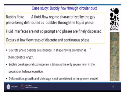
So circular duct we are having bubbly flow. So here the discrete phase we have using population methodology and deformation growth and shrinkage we have not considered in the present model okay. So breakage and coalescence we have considered using your population balance methodology. So let us see over here as we will some results.
