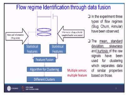
So ring kind of wall probe is nothing but a circular ring attached with the inner wall of the tube okay. So 2 rings we have given like then from there we have obtained the signal. And here these are actually diametrical wires. So these actually, these 2 wires are actually in 2 strip types so actually restricting flow path. But these are actually wall attached okay wall attached ring kind of probe so these are not restricting the flow path.
