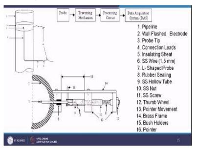
So this conductivity probe is having trade in type of active probe, also we are having a central probe which is kind of you know round so we will be taking signal between this ring type of probe and this central probe. And the cross sectional view we have shown over here. So this is your pipe section so along this we have a fused ring type of probe.
