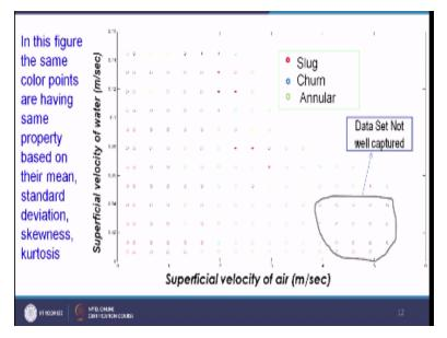
Now here all these points are identified based on the clusters as we have mentioned in the previous slide you say different clusters. So we have actually fused the signals obtained from this ring probe and parallel wire probe and finally we have found out 3 clusters cluster for slug flow, cluster for churn flow and then cluster for annular flow.
