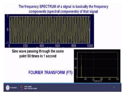
You see basically here in this plot you can find out this is time okay. And here we are having some data and this may be some probe signal, optical or electrical conductivity probe or some other type of probe signal. So here let us consider that we are getting the signal. What I have shown you over here, this is actually a sine wave you can see it is showing sinuous nature okay.
