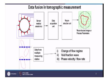
So we are having here optical sensors in the periphery of the pipeline. So lots of optical sensors we have given in the sector you see and all the signals are actually coming out over here in the readout. And then from the readout we are going to data acquisition system and finally reconstruction is being done for the interface.
