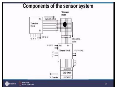
So you can find out that this vertical wires whatever we are having those are coming from the receiver circuitry. And whatever horizontal wires you are having those are coming from transmitter circuitry. So power is given to this 1 okay. Now what you can do at each cross point you can find out the voltage. As you are having a mesh kind of structure so from the mesh structuring at every point you can find out the voltage.
