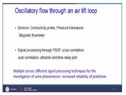
Here in this experiment you will be using conductivity probe signals pressure transducers and magnetic flow meters okay. And for signal processing you will be using PSDF, Probability Spectrum Density Function, cross correlation, auto correlation, attractor and time delay plot. So as we you have already understood this is having conductivity probes having multiple sensors over here.
