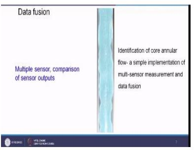
So this is actually liquid liquid core annular flow, a figure I have shown you over here this is the kerosene figure okay kerosene and air. In the annular domain, you see here we are having the white portions these are actually water. So, this is liquid core annular flow and the liquid, liquid pale is kerosene and water. So, let us try to see that whether we can capture this annular flow using, you know multiple sensors and if you compare the signals between the sensors okay.
