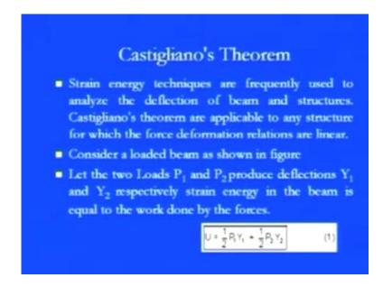
So, coming to the strain energy technique frequently used in, you know like, analyzing the deflection of beam and the structure as we discussed. So, Castigliano's theorem are applicable to any structure for which the force deformation relations are linear. So, that is what, you see, I told you that if within the elastic region, if any slight change is there we can simply go with this particular theorem.
