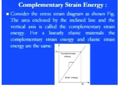
So, consider the stress-strain diagram as shown in this particular way also; the area enclosed by, you know like, the inclined line and the vertical axis is called as the complementary strain energy. And for linearly elastic material, the complementary strain energy and the elastic strain energy are same.
