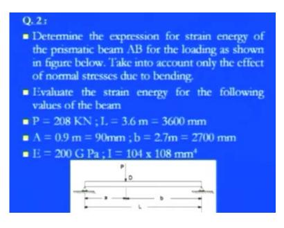
So, determine the expression for the strain energy of a prismatic bar AB for the loading conditions as shown in this particular figure and taking into account only the effect of
