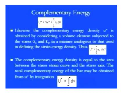
So, come to that point U star and I told you that the W star, which is the complementary work is there, is responsible for complement strain energy is equals to zero to P because, you see, that a limiting load is P, so zero to P delta 1 into dP.
