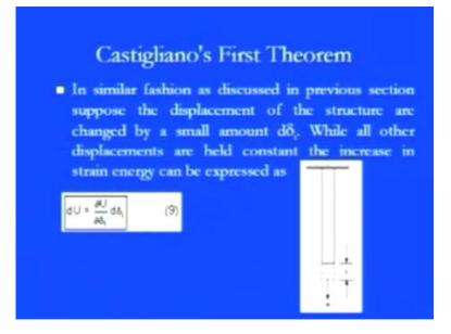
In a similar fashion as discussed in the previous section, the displacement of the structure are simply changed by small an amount of this delta d delta. While another, you see, the displacements are simply, you know like, held constant and there is an increase in strain energy is there which can be simply expressed by dU is equals to del U by del delta into d delta.
