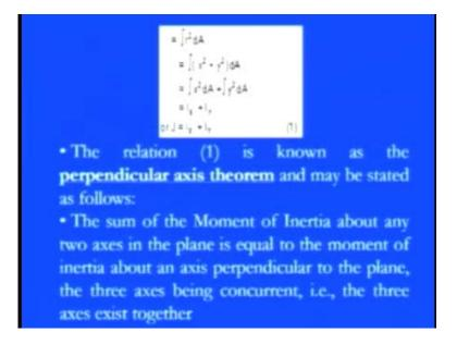
So, for that matter you see always whatever the second moment of area is coming, the new term is there for that which is the J which is also known as the polar moment of inertia, and it can be you know like calculated because it is just focused on this. We have the R of the distance for that which I have shown you this R distance from O to our elemental area. So, this integration of R square dA will be equal to J or since, R is nothing, but was you see x and y was there.
