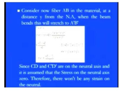
Now, you see consider the fiber AB of the material, you see as I told you in the intermediate section, if you are just focused on the fibers of that particular path of the AB line at the particular distance y from the neutral axis, then the bend will be stress to A
