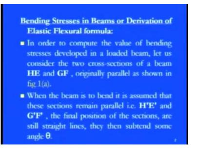
So, in order to compare the value of bending stresses developed in a loaded beam, first of all we need to consider the two cross-sections of the beam like HE and GF originally parallel because there is no bending moment and then they are absolutely parallel to each other.
