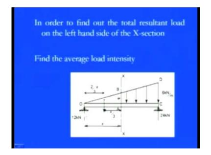
So, in this figure, you can easily visualize that, kind of part that, at this point, since it is w; w is equals to x by 2 is loading and it is locating at this particular point. So, two-third of x is there or we can say one-third of x is there. So, we can find it out that, how shearing will be occur at this due to this particular diagram. And then we will extend beyond this particular reason.
