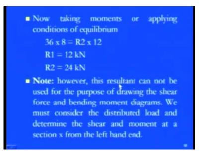
So, now, with that, we can easily calculate that remaining reactions. So, 36 into 8 from one end is equals to R 2 into 12 by taking moment at this particular junction R 1. So, we have this R 1, which is 12 kilo newton; and R 2, which is 34 kilo newton. There is one note. However, the resultant cannot be used for the purpose of drawing shear force and bending moment diagram.
