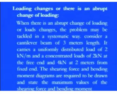
So, when there is a abrupt change of loading or load changes, the problem may be tackled in a symmetric way. Just total... means the same system is there; there is no change in that way whatever the symmetricity, which we have assumed. Again the same systematic pattern is there in that way also. So, if we consider a cantilever, now, just take
