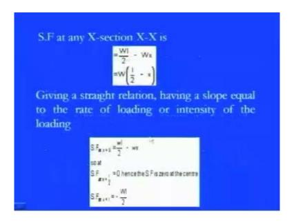
The reaction forces are and then at XX cross section the shear force is W l by 2, because of the reactions the this particular reaction which is going upward direction and you see the middle portion W into x is there which is the total intensity of the load into x. So, this will go in the downward direction, so we have a positive side here W l by 2 minus W x are we can say, if you take the W common then we have l by 2 minus x.
