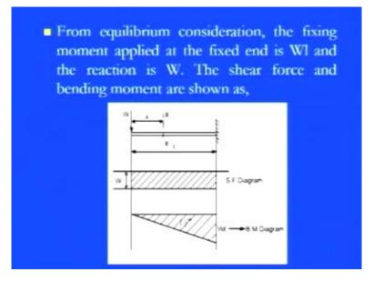
So, from the equilibrium consideration the fixed movement applied to this fixed end, because you see we have cantilever. So, we have a fixed end, which is equals to whatever the bending moment is there, W into I and reaction which is due to the shear force is W. So, come to that point, what we have this cantilever, so the cantilever is this one, this is the rigid end, this is you know like the free end and as I told you know like we have a point load at the extreme corner of the free end.
