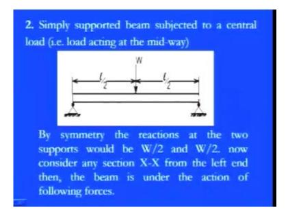
This is a simple, the uniform cross sectional beam, these two supports are there and when we apply the point load at the mid section, you see 1 by 2 in 1 by 2; that means, you see we have the total cross section at the total length of beam is 1. So, by the symmetricity is there, because the point load is at the centre point, the reactions are coming at extreme corner the length is 1 by 2, 1 by 2.
