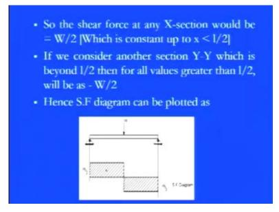
So, by considering that concept, what we can do here we can simply find it out, that what is the magnitude of the shear forces at the cross action, that would be always W by 2 which is constant up to X is less than 1 by 2. Because, after X equals to 1 by 2, we have additional W, so you see it will add up in that particular part, so now we just want to see that, what will be the shear force diagram.
