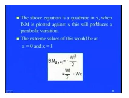
In terms of say, I told you and bending moment is plotted against x, this will produce a parabolic relation, so as I told you it is not straight relation, it is now a parabolic relation. So, x square equals to 4 a y, so staring from x equals to 0 to x equals to 1, if you are keeping x equals to 0; obviously, there is no bending moment at that particular point. If
