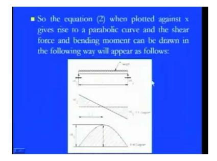
So, if you keep those things, then you have minus W l square by 8, so by summing up of all the relations, we have pretty simple diagram first of all the shear force diagram, these two reaction force W l by 2, W l by 2. So, we have the positive W l by 2 in this way, because it is going in this direction and then it is in this direction this one, so it is a negative direction and variation is this, so plus W l by 2 to minus W l by 2.
