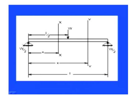
So, see now considering the same part, you see we have this, 1 length same cross sectional beam, these reactions which have the same magnitude W by 2, W by 2 and acting towards the upward direction. And, you see this point load is there, which is just acting downwards and because of that we have the shearing action in this portion as well as in this portion also. So, in that if you go for the left hand portion you know like what we are doing here we are first considering the X x portion.
