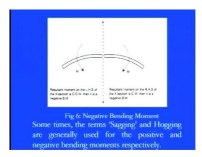
And due to the resultant of all these forces on a beam, if they just tend to move in anti, with this, you see in the left hand side if they are just moving in a counter clockwise direction and the right hand side, if it is moving in clockwise direction. To balance those things if we have the tendency of the total beam in this direction, we can say, that this is the negative bending moment.
