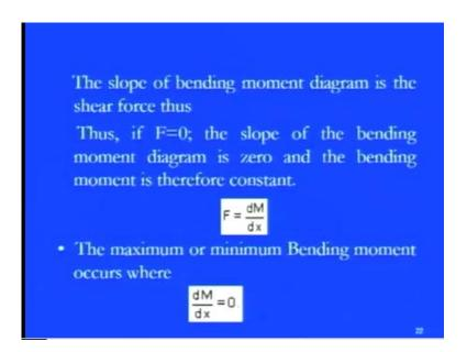
The slope of bending moment is nothing but the shear force; that is the key part. If you, if you know the slope of the shear force, that means, if you have the value of M and if you just take the slope of that, you have the value of the shear force. Means, you see, if we have F equals to 0 that means, the slope of bending moment diagram is 0. The bending moment is nothing but the constant.
