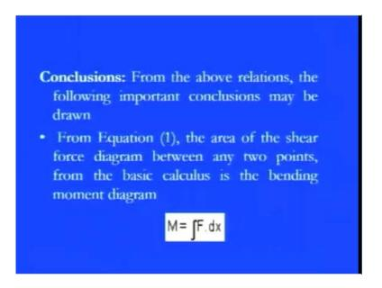
So, now we would like to conclude that part. From the above equations, whatever you see, the two equations, the following important conclusions we can simply drawn. First, the equation was, which, which was correlating the shear force and the bending moment. So, from the equation 1, the area of the shear force diagram between two different points
