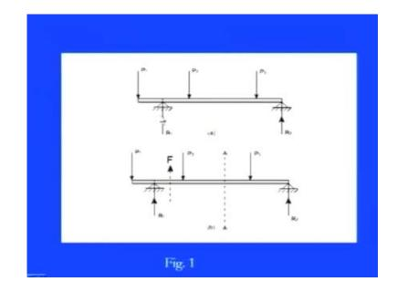
So, now our main thing is just to consider the beam, you know, like as shown in this figure, that we have a beam and in this beam we have the two supporters. So, here you see, this beam, which is having the length l is supported at these two corners. One is the overhang part is there, so this end is free and it is supported by that. So, this is the overhang portion and this is exactly supported at the end.
