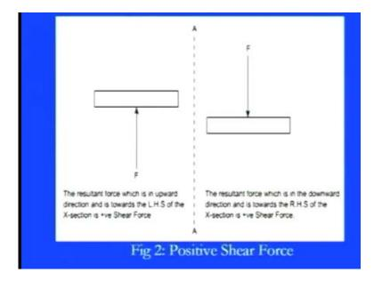
So, our first focus is, that what is the sign conventions are there for these kind of shearing forces? So, you see, the usual sign conventions, we simply categorize into two main figures. So, figure two is simply showing, that if we have the resultant force on left hand direction in upward direction. That means, you see, the resultant force, which is upward direction and towards, you see, the left hand side of any cross-section is a positive shear force.
