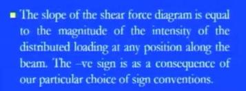
And then you see, you know, like the last part the slope of a shear force diagram is equal to the magnitude of the intensity of distributed loading. Just keep this thing in mind. And whatever the slope is there, you see, of the shear force diagram, because the slope of the bending moment will give you the shear force, but the slope of a shear force will give you the magnitude of the intensity of the distributed loaded at any position of the beam.
