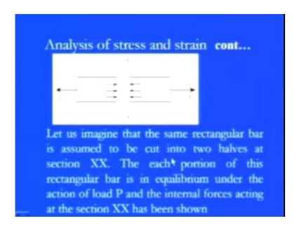
So, if you want to analyze those things, first we need to make the cross section and that is why you see you know like in this, then this diagram we are shown here that there are two main parts and on both of the sides, both of the end sides here, the P external excitation force is there and due to this externally applied load. We have seen that if you cut those thing at both ends through this XX line, these internal resistances are there.
