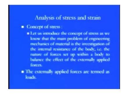
As we know that the main problem of engineering mechanics of material is the investigation of the internal resistance of body because you see you know like if we apply the load, always body will react by the third law of the this Newton that the reaction you know like action reaction is there. So, as you apply any kind of load, whether it is a uniaxial, biaxial or triaxial load, always a kind of resistance will take
