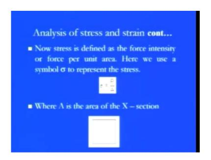
If you are talking about the analysis of the stress or strain within those things, we can say that the stress is defined by the force intensity or the internal resistance force is per unit area. And hence, we use the symbol sigma just to represent the stress, that is P by A, where A is the cross-sectional area here which is the rectangular area is there because the rectangular bar we have used in the previous case.
