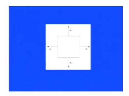
So, these are nothing but, the along this principle strains component, so here you see we have this unit cube and these two mutually perpendicular stresses are there and we can easily represent in this particular unit cube. So, we have you know like the unit cube in which we have unit depth, unit height and unit width is there, so along that in the x axis we have the longitudinal stresses and due to longitudinal stresses we have you know like the longitudinal stress.
