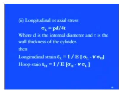
And we have the another component that is the longitudinal strain or the actual the stresses are there that is nothing but, the p d by 4 t, where the d is the diameter and t is the wall thickness of the cylinder. And corresponding you see you know like we can compute that how much deformation is there, in these corresponding direction, so we have you know like the longitudinal stress was there.
