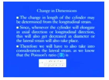
So, if we discussing that when there is you know like, the flow is flowing in the thin cylinder and change in length is there of the cylinder along that path, then definitely you see we have along the path of the longitudinal direction, then we will be having a longitudinal deformation. And if you want to measure the longitudinal deformation; obviously, you see the longitudinal strain is the main component through which, we can say that how much deformation is there.
