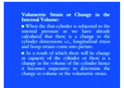
So, now again first thing will come that what is the volumetric strain or due to the changes you see because, if there is change in the length, direction or the longitudinal direction, then there is an impact of the this the diametrical way. So, what exactly happening with the total volume, so now you see for measuring those that what the net change is there in the volume, if you want to measure that kind of deformation, always you see there is a strain component.
