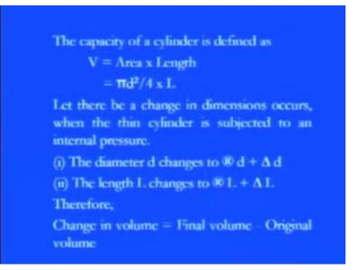
And now you see would like to you know compute the volumetric change, so the capacity of cylinder is nothing but a the area into the length and since you see we are considering the cylinder. So, area is pi d square by 4 along the length into since you see here we are considering that actually along the length what will be the area. So, area is pi d square by 4 into L and let there be a change in the dimension occurs along the length when a thin cylinder is subject to a internal pressure.
