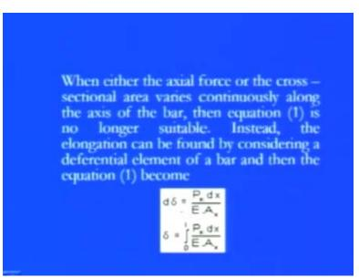
So, we will see here the d del which is nothing but equals to P x dx divided by E times A x. Meaning is pretty simple that if we have a small segment even if it is the tensile loading is there, it can be easily you know like the load applications are there in the axial part because it is a uniaxial loading is there. So, P x is there, and then you see whatever the small segment is there that is the dx segment in terms of the area A x is there in terms of Young's modulus we have E.
