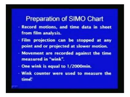
And time data in study sheet from the film analysis, in the film projections can be stopped at any point or projected at slower motion and movements are recorded against the time measured in wink, wink is a time unit which is used for recording the various therbligs and this wink is very small one wink is equal to 1 is 2000 of a minute 1 by 2000 of a minute.
