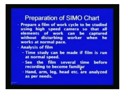
For preparing the SIMO chart film of the work cycle is prepared first and that is studied and that film is prepared using the high speed cameras. So, that all elements of the work can be captured without disturbing the worker, so this first step for preparing the SIMO chart the film of the work cycle is captured in such a way that no element of the work is lost and this is done without disturbing the worker when work is being carried out at normal pace.
