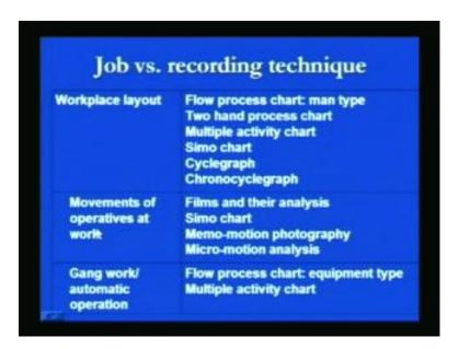
The other objectives like the kind of workplace layout study or it is optimization of the plant layout. The movement of the operators at work, means the kind of the way by which the body parts and the individual body parts movement is taking place or the way by which operator is moving during the operation or the in gang work, where number of workers are working during the operation or one worker is looking after the number of a automatic machines.
