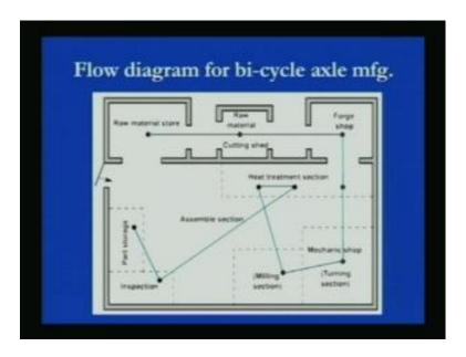
As I have said that flow diagram shows the top view of a the department or the section where work is being done, indicating the different stations where work is carried out. And also shows the different points, where points which can affect the extent of movement of the worker during the operation, for example here this is an example related with the manufacturing of bicycle axle manufacturing, material is taken for the stores and then it is moved from a stores to the cutting section.
