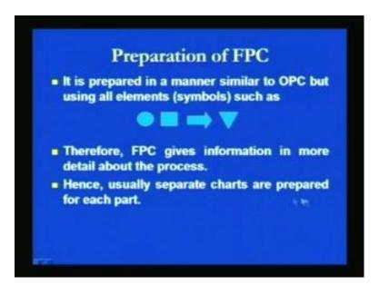
The for preparing the flow process chart, these are the symbols which are commonly use like operation, inspection, transport and the storage. Delay is also used where material is kept under the unauthorized conditions, like waiting of the material for further processing. It is prepared in a manner similar to the Outline Process Chart, that is called OPC, but using all elements in form of the following symbols.
