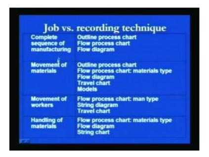
So, here if you see the recording techniques can be used for the different purposes like, study of the entire sequence of the manufacturing of a particular product or to study the movement of the man or material during the operation, to study the movement of the worker to investigate, the handling of the material and likewise various other objectives. Depending upon the kind of objectives, the specific kind of process chart can be selected depending upon the range of operation also.
