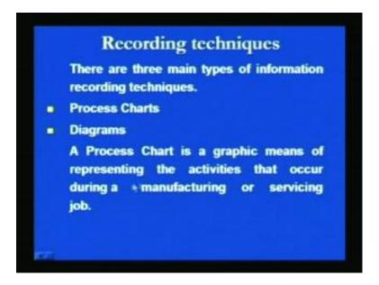
The charts and the diagrams are very extensively and commonly used to record the events and activities, ranging from the entire plant to a particular department. The process chart is defined as a graphic means of representing the activities, that occur during the manufacturing or servicing of a job.
