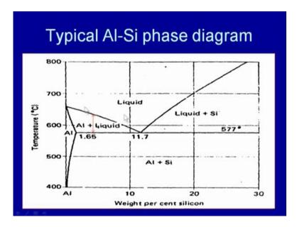
For example, if we see here, this is the liquidus line and this is solidus line in case of the aluminium silicon phase diagram. When aluminium is pure, it solidifies means, the melting and the solidification temperature is one and that is around 662.5 degree centigrade. And with the addition of the silicon, we can see there is the range of the solidification temperature keeps on increasing and for about say 1.65, the solidification temperature range is maximum.
