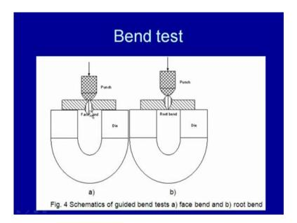
So, in this case very guided bend, the die is used and the load is applied from the top and above the die the weld joint to be tested is placed. In this case, the face will be subjected to the bend when the load is applied and we keep on applying the bending load until the cracks start to appear on the surface which is being bent. So, here in this case the face
