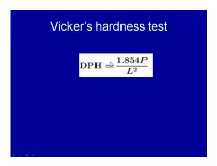
Indicating the diamond pyramid hardness number or it is also termed as the Vickers hardness number, is obtained from the 1.854 P, P is the load applied and l is the average
