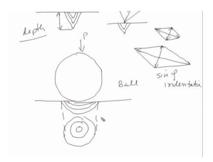
So, lower is the depth or lower is the size of indentation, means lower average length of these diagonals, that will be and. So, lower is the depth or smaller is the size, average size of these diagonals these will be, indicating the higher hardness. Similarly, for the
