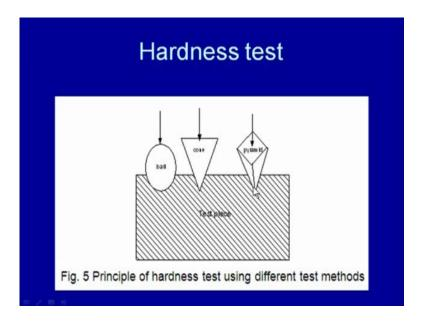
And this is the example say in case of the ball; the indentation is taking place like this. So, the indentation diameter is measured at the surface, in case of the cone here, the depth of indentation is measured and the average length of the diagonals is measured in case of this pyramid shape indenter. And in all the cases say the extended load is applied and then the extent of damage at the surface is taking place in terms of that indentation, that is characterized to measure the hardness.
