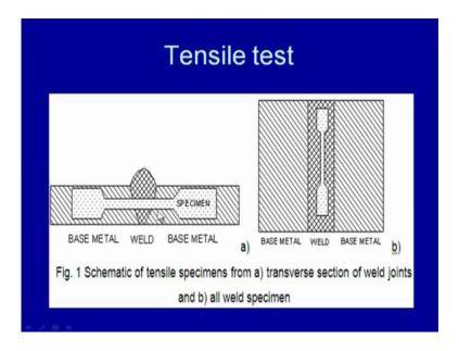
So, say this is the case when the weld the tensile this is the plate, with the weld joint, this is the weld region and the sample is obtained from the transverse direction of the weld this is the weld centres say. So, the specimen is being taken from the transverse direction of the weld. So, here at the centre of the weld we will be having centre of the specimen we will be having the weld region.
