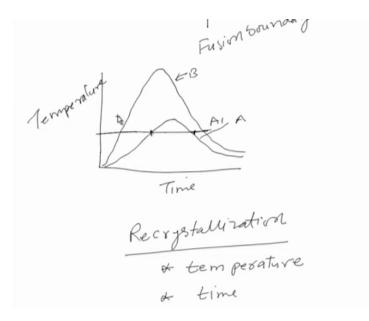
Then the weld thermal cycle corresponding to the location b will be like this which is closure to the fusion boundary and that of the location which is away from the fusion boundary will be experiencing lesser temperature. So, if this is the critical temperature so the soaking time and the temperature. If we see the exposure above the critical temperature that is say A1 will be for shorter period for location a.
