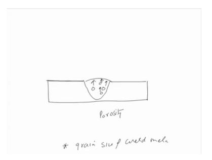
If we have this weld and here we have the gas packets in the dissolved state if the solidification of the weld metal is occurring fast, then this gases will not be able to come out of the molten weld region. So, this will be interrupt and will result in the porosity. Similarly, this can be inclusions, which can be formed due to the interaction between the different elements present in the weld metal or a reaction between the gases present in the arc environment and the metal in the molten state.
