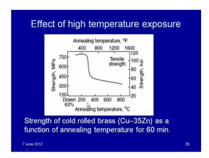
So, depending upon the metal system the different the temperatures are required for the recrystalization. If we see here if we give an exposure to the metal system at the different
