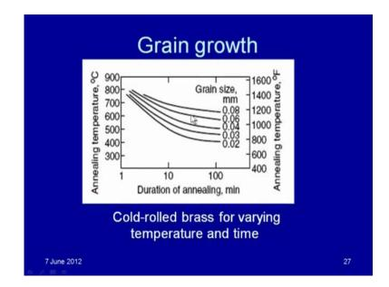
So, we know that if the both exposure temperature and the time significantly affect the grain size. So, if we take up again the case of the cold rolled brass for varying temperature and durations, then simply reduction in the exposure temperature helps in a decreasing for identical time helps in decreasing the grain size or for the given a exposure temperature, increase in the duration increases the grain size. So, these different lines are corresponding to the different grain sizes.
