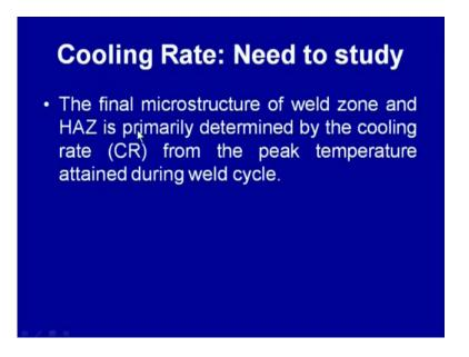
So, if we see here the final structure of the weld zone and the heat effected zone in the weld joints is primarily determined by the cooling rate, which is being experienced by them from the peak temperature during the welding, so if we have to see this we can see this in the next diagram.
