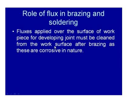
The fluxes are applied over the surface of the work piece for developing the joint must be cleaned from the surface of the work piece after the brazing because these fluxes present on the surface of the work piece are found to be corrosive in nature. Therefore, once the fluxes are applied these must be removed from the surface. The fluxes which are commonly used for performing their role means reacting with the impurities and removing them in form of the slag.
