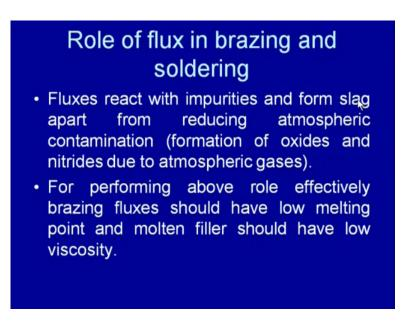
So on melting, these filler material the fluxes helps in reducing surface tension of the molten filler material, which in turn helps in improving the wetting action and increases, which in turn increases the spreadability or the ease by which the molten filler material can get distributed between the faying surfaces. And further, it protects base metal and
