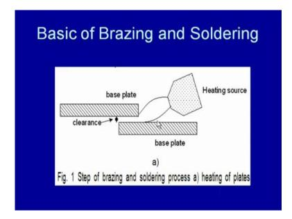
So, here we see the arrangement is the red plates are kept under the, in a particular position with the controlled gap and the heat is applied using a suitable heat source and then filler material is placed near the edges of the plates to be welded are to be joined. And subsequently on melting of this filler material it gets distributed by the capillary action between the, in the gap between the members to be joined.
