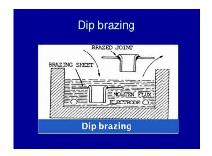
Alternatively assembled joint parts are dipped in the molten metallic bath, so that the joint can be made. And the molten metal in the bath fills the joint. So, the assembled
