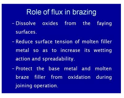
These fluxes basically dissolve the oxides from the faying surfaces and reduce surface tension of the molten filler material in order to increase the wetting action and the spreadability. So, when the fluxes are present and heating of the filler material is done.
