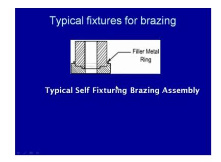
This is the situation where the filler material is, between the two components filler material is placed and then this entire assembly is passed through the heating furnace. So, in this situation like self fixturing brazing assembly here the filler material is placed between the components to be joined and then it is passed through the furnace and after that on solidification we get the braze joint.
