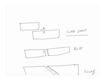
For developing the weld joint, for developing the braze or soldering, solder joint it is necessary that the plates are cleaned first. And the all the impurities, oxides, oil, grease etcetera present on the surface of the plates to be join is removed. So that the proper capillary action can be obtained for uniform distribution of the filler material being applied at the edges of the plates to be joined.
