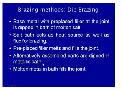
In the dip brazing the base material with the pre placed filler material at the joint is dipped in to the molten salt bath for applying the heat onto the component. The salt bath acts as a heat source as well as the flux for the brazing. It avoids any atmospheric contamination of the molten filler material during the joining and in the pre placed filler material melts and fills the joint.
