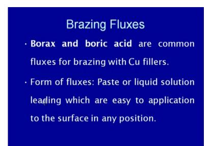
The borax and the borax flux or the boric acid, are commonly used for the brazing with the copper filler metals. And these fluxes can be used in form of paste of the liquid solution which can be easily applied at any position during the joining process. For the brazing depending upon the source of the heat which is being used for heating the base material for developing the braze joint the various brazing methods have been developed.
