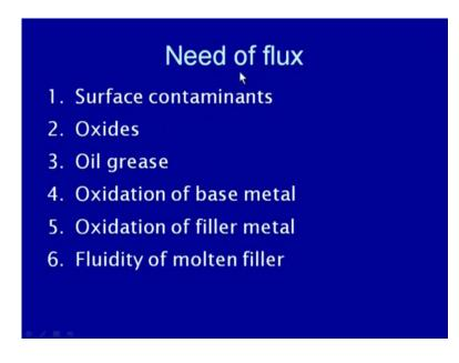
So, in order to remove them the fluxes are used as they will dissolve the impurities present on the surface and to may, will make them clean. Further, these will also dissolve the oxides present and prevent the further oxidation of the base material. So, after removing the oxides present at the base metal surface the further oxidation is removed, reduced by, prevented by the fluxes when they are used. The fluxes also helps in removing the oil and grease which is present on the surface.
