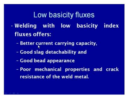
Basicity of the flux in the submerged arc welding affects the variety of the characteristics which are important in developing the sound weld joint; these are the current carrying capacity, the slag detachability. How easily we can remove from, how easily the slag can be removed from the weld bead the shape of the bead, that is the reinforcement and width of the weld bead and the mechanical properties and the cracking tendency of the a weld joint.
