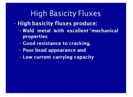
So, when we use on the other hand the high basicity fluxes these fluxes offer the weld metal with very good mechanical properties due to the reduced impurities and oxygen content in the weld metal and cleaner weld metal is produced. This in turn results in the better mechanical properties at the same time good resistance to corrosion cracking is also observed, but the weld bead appearance is poor and the current carrying capacity is also reduced.
