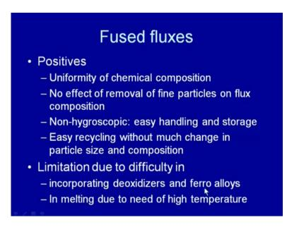
So, that the desired combination of the properties can be obtained in the weld metal the fused fluxes are the one, where we will be taking up the first the positive sides of the fused fluxes. The important thing with the fused fluxes is that the uniformity in the
