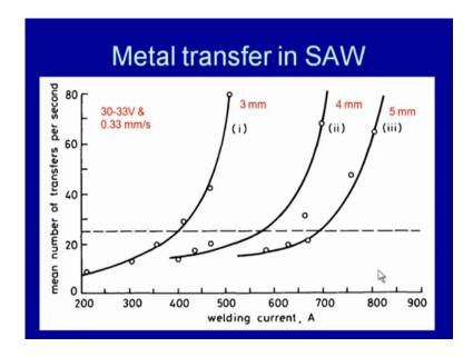
Now, we will see that the transfer of the molten metal from the electrode tip to the weld pool in the submerged arc welding. We know that a the metal transfer is a very is an important phenomena in the consumable arc welding process where electrode tip melts and the molten metal is transferred to the weld pool during the welding. It can happen in number of ways like short circuiting transfer, globular transfer, spray transfer, rotational transfer and explosion etcetera.
