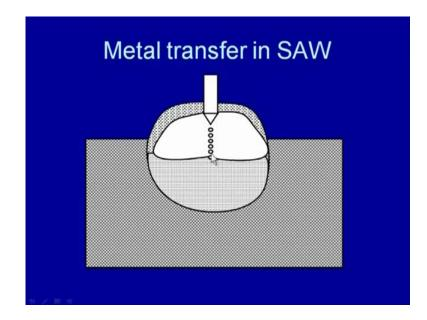
When the droplets are of the very small size, very frequent formation and the detachment can occur during the welding. So, transfer of the molten metal from the electrode tip to the weld pool can occur in the different ways in the submerged arc welding.
