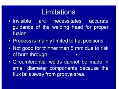
This process also suffers with the certain negative points like arc is invisible say it necessitates the accurate guidance of the welding head for proper fusion of the base metal along the weld line. This process mainly limited to the flat positions because it is required to form a pool of the flux around the arc and other than flat positions like in vertical horizontal and overhead it becomes difficult to have this kind of pool around the arc.
