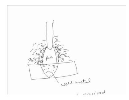
So, these elements are mixed in form of powder with the flux and when this flux melts during the welding these powder particles also melts and they get mix up with the weld material. So, this approach for modifying the composition of the weld material as per requirement is that the mixing of the required elements with the flux itself.
