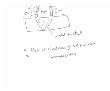
To change the composition of the weld metal there are two possible approaches, one is use of electrode of required composition. This is one, but sometimes it becomes difficult to get the electrode of the required composition. So, under such situations where it is not possible then we can use comparatively unalloyed electrode material and the required elements can be added in that case while putting the elements with the flux.
