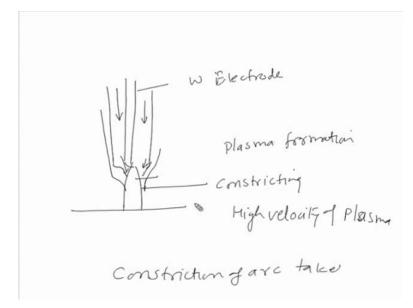
First, we use one tungsten electrode and then this tungsten electrode is used to establish the arc. So, this arc can be established either between the base material and the tungsten
