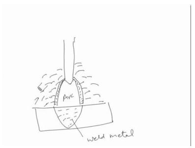
So, this approach is very simple if we have to understand this we will see this schematic diagram where we can see that this is the electrode and this is the welding arc. This welding arc is completely covered by the flux all around and or a thin layer of the flux is brought to the molten state. So, this is molten layer, the layer of the molten flux around the arc and this is the arc zone and here we have the weld pool. So, to change the composition of the weld metal this is weld metal.
