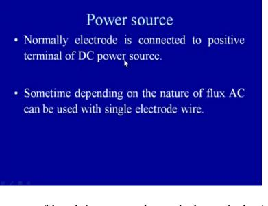
So, that more amount of heat being generated towards the anode that is the positive terminal side of the electrode can be effectively used for fast melting of the electrode and so has to achieve the higher deposition rate. So, the high deposition rate can be obtained while making the DCEP that is the electrode positive polarity. But when DCEN is used it results in the shallow penetration in the weld.
