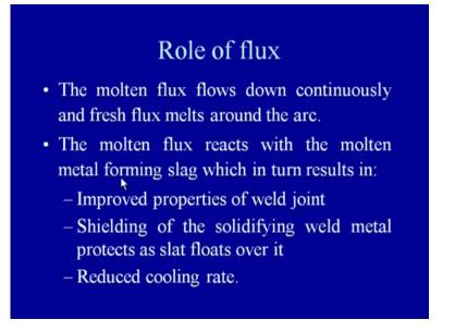
So, because of the reaction of the molten flux with the impurities present in the weld metal, the these impurities are take of at the removed by the flux which in turn helps in improving the properties of the weld joint. And it provides the shielding of the solidifying weld metal to protect it from the, to protect it from the atmospheric gases.
