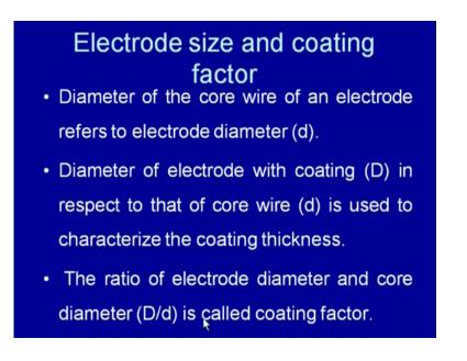
Now, we will see that what are the factors that are used to designate the electrode, and identify the electrode size. What is the coating factor which is indicating, the thickness of being used for developing thickness of the flux or the coating being used for developing
