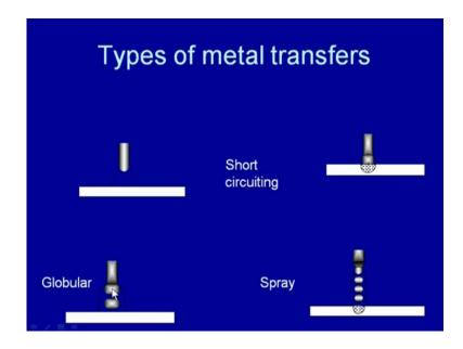
So, depending upon the kind of contamination electrode coating composition we can have short circuiting transfer globular or spray transfer. So, in short circuiting transfer is observed when the molten metal drop grows to such an extent that it touches to the weld pool short circuiting takes place and then it gets transferred. While in case of the globular transfer the drop gains to such a large size that even if the diameter of the drop is greater than the electrode diameter.
