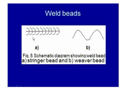
So, this is what we can say the stringer bead is shown and the weaver bead when different patterns are used for developing the beads. Weaver bead helps to apply more amount of heat in per unit length during the welding.
