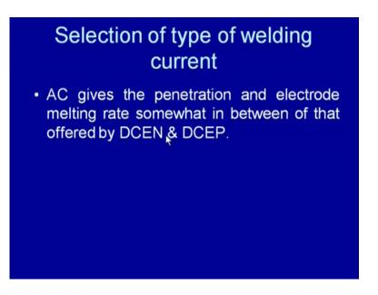
AC gives the penetration and the electrode melting rate somewhat between to that of the DCEN and the DCEP. So, if the control over the heat input is not a very important factor for developing the sound weld joint then AC is preferred. Provided we are able to have the smooth and the stable arc for producing the uniform heat.
