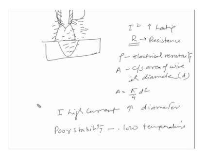
So, we have a cross sectional area of the wire from the pi by four d square, where d is the diameter of the core wire. Larger is the diameter greater will be the cross sectional area and if greater is the cross sectional area lower will be the resistance for the flow of current. So, if by using the large diameter electrode we are able to reduce the resistance
