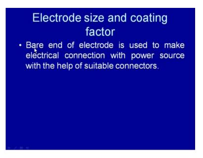
So, greater is the length of the electrode lower will be the current carrying capacity of the electrode for a given diameter of the core wire. Further one end of the electrode is not coated with the material and it is kept bare, so that the suitable electrical connections can be made with the power supply for required flow of the current. Now, these electrodes need to be classified so that one can use them effectively and one can select them properly.
