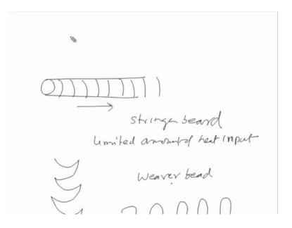
For example, if we want to deposit the weld bead with very limited amount of heat input then stringer bead is preferred. But if we want to use the lot of heat to deposit the weld metal we want to apply more heat more, and more amount of heat during the welding then the weaver bead is used. This weaver bead is commonly used when we are working in a odd position.
