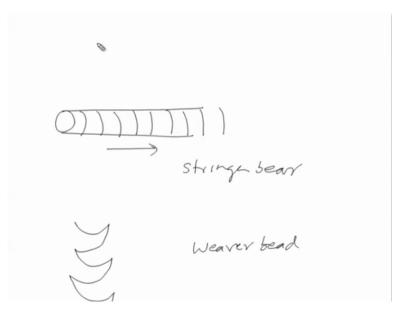
So, especially this in case of this stringer bead the weld metal is allowed to deposit in the straight line like, this one and not much movement is given to the arc and the electrode. So, this one is called a stringer bead. While in case of the weaver bead the arc is manipulated in different ways and these manipulations may be in different forms like one is like this. These are the different paths through which we can keep on moving or...
