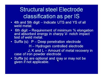
Further the fourth and fifth digits indicates basically set of the three numbers which indicate the ultimate tensile strength and the yield strength of the weld metal. So, set of the three digits a forming the combine combining ((Refer Time: 32:36)) and the fourth number indicates the ultimate strength and the fifth digit indicates the yielding strength of the weld metal. Sixth digit indicates the requirement of the minimum percentage
