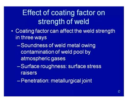
Weld bead coating factor effects the strength of the weld joint and this effect of the coating factor on the strength of the weld joint can be understood in the three ways. One is that how the coating factor is affecting to the soundness of the weld joint, the second
