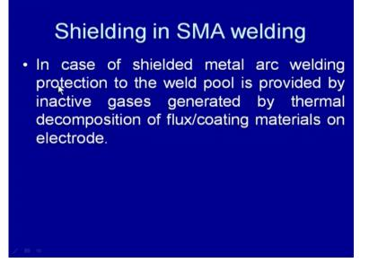
So, in case of the shield metal arc welding process protection to the weld pool is provided by providing the inactive gases around the welding arc. These, inactive gases are generated by the thermal decomposition of the flux, which is present in form of the coating material on to the electrode.
