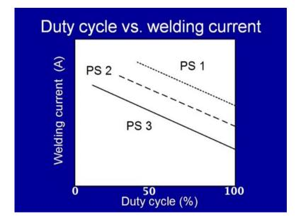
So, in general, if we are drawing the higher current then we need to work with the lower duty cycle. For example, if we see here y axis shows the welding current that we can draw and x axis shows the duty cycle at which we can work at 100 percent duty cycle. We can draw very low level of current for a given power source and this varies linearly, if we keep on decreasing the duty cycle. Then the welding current at which we can work will keep on increasing.
