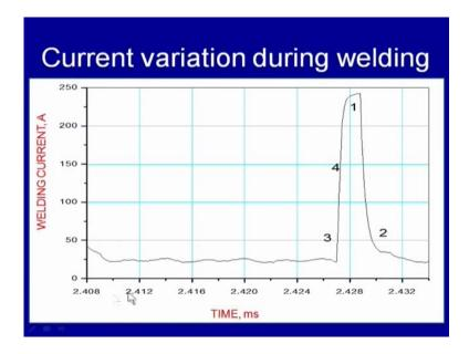
If the kind of transient conditions, which are experienced during the welding we can say there is a sharp change in the welding current over a period of a say very short period of time. Say it increases suddenly, then it comes down and passing through the different stages of a. Due to the fluctuation in arc length and the changing welding conditions. Similarly, here we can see that the how arc voltage fluctuates during the welding over a very short period of the time.
